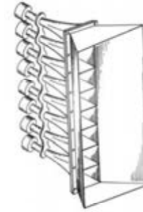
re 16-77 Whelen Engineering horizontal diffraction horn with multiple drivers. (Courtesy Whelen Engineering Co., Inc.)
