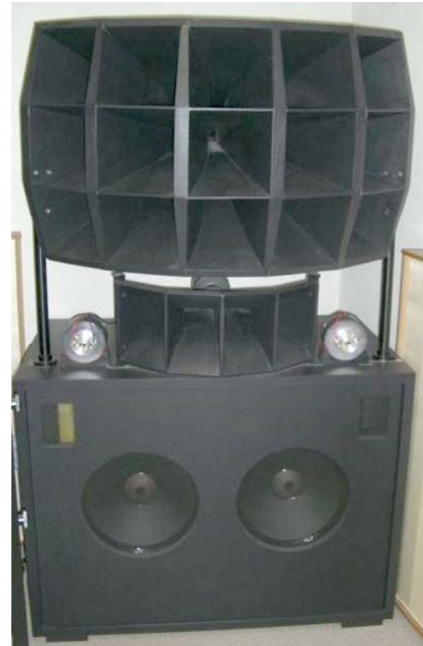
Onken 255 wood and Onken 455 wood horns on top of an Onken W bass reflex enclosure
