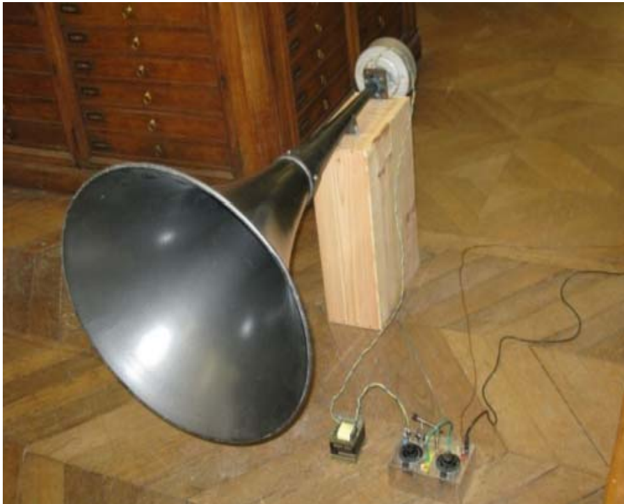
my home made crystal radio with a Vitavox E190 horn
