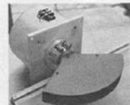
Fig. 2. The tweeter resembles an ordinary high-frequency speaker except for the relatively large field coil housing.
